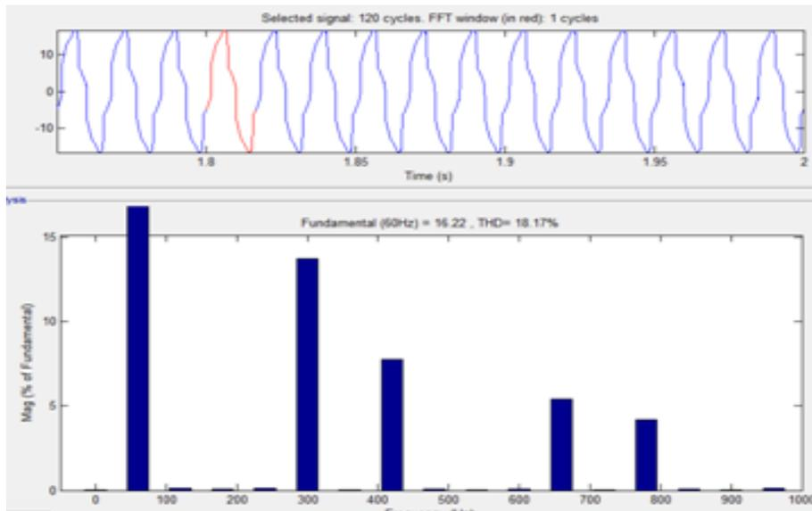
Load current total harmonic distortion (THD) Without controller is 18.17%
