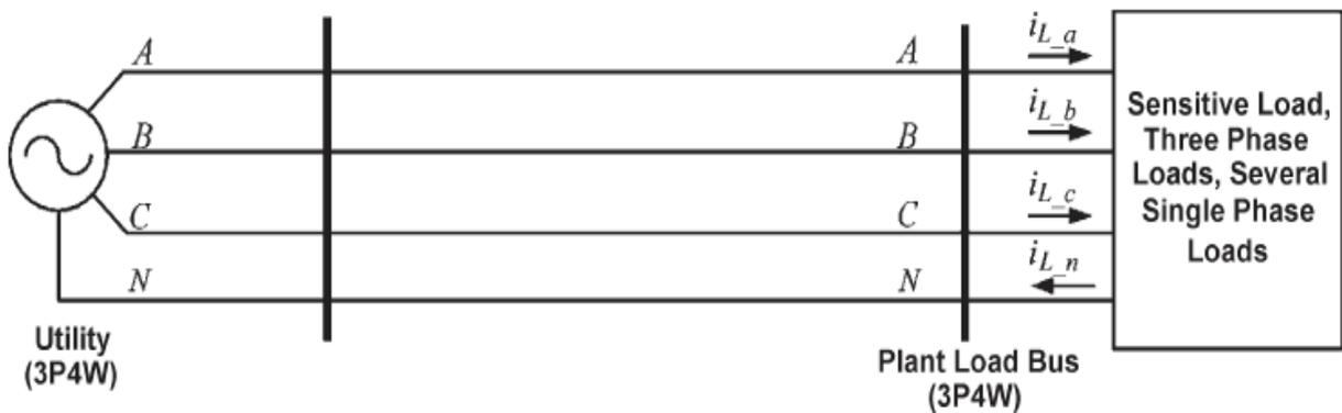
Fig. 1 3-phase four wire distribution system (Neutral is provided by generating station)
