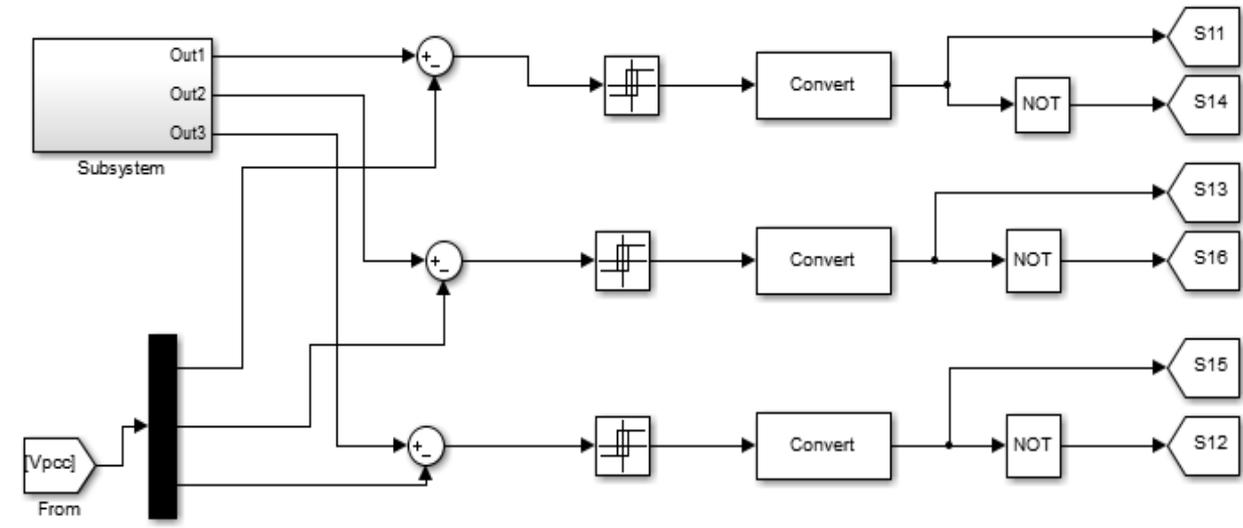
Fig: Matlab model of Series active power filter
