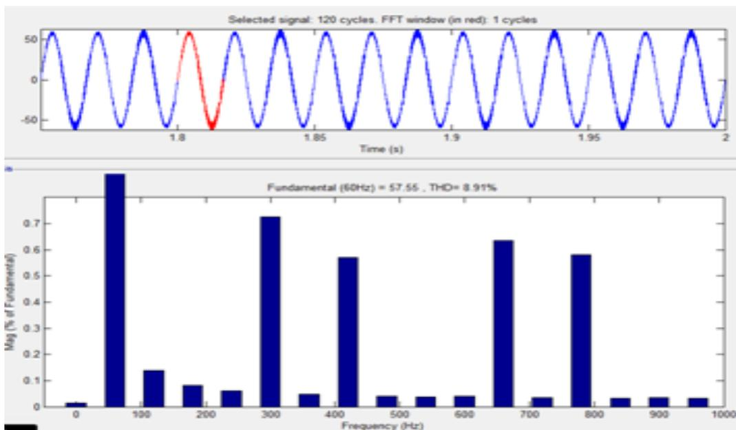
Fig: (I) Load voltage total harmonic distortion (THD) Without controller is 8.91%
