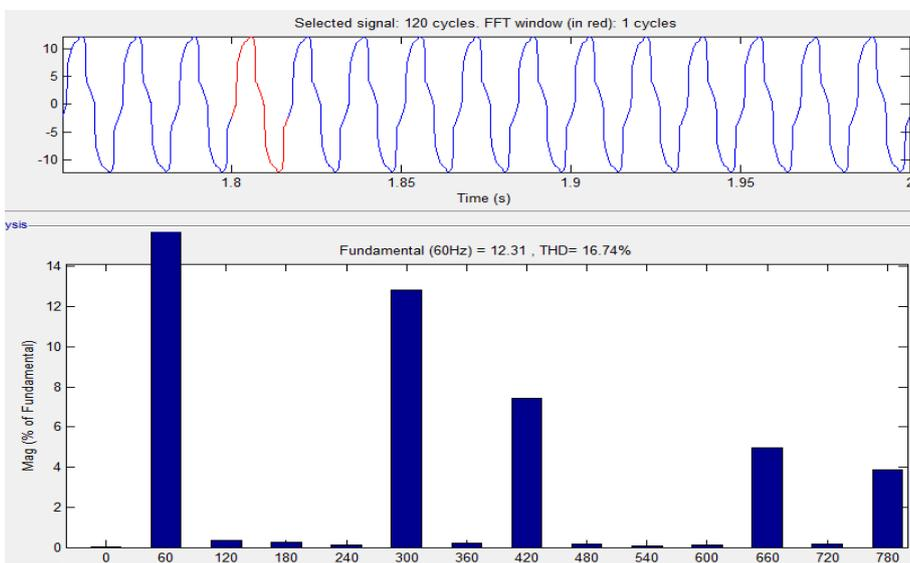
Load current total harmonic distortion (THD) With controller is 16.74%
