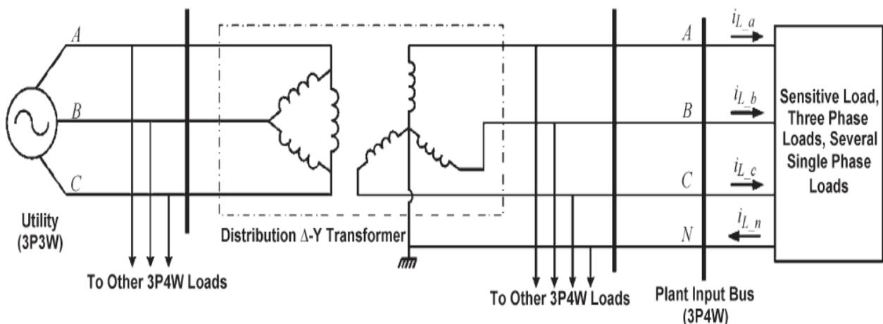
Fig. 2 3P4W distribution (neutral is provided by  $\Delta$ -Y transformer)
