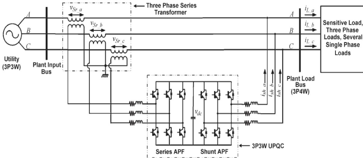
Fig. 3 3P3W distribution system with UPQC
