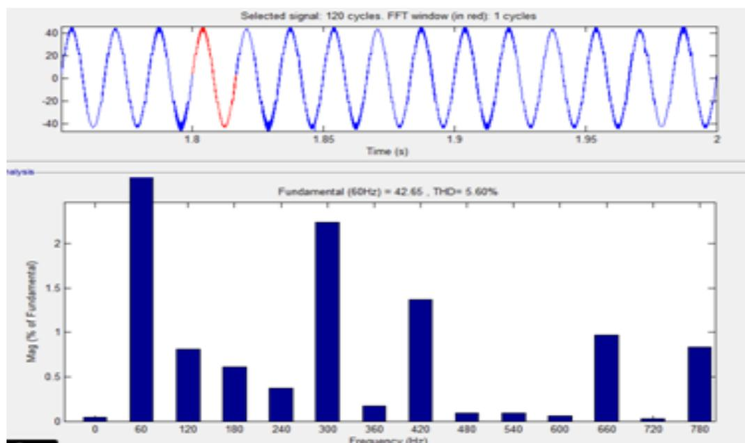
Fig: (j) Load voltage total harmonic distortion (THD) With controller is 5.60%
