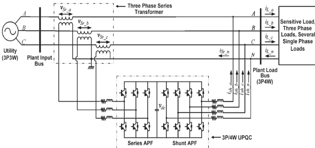
Fig. 4 3P4W distribution system with UPQC
