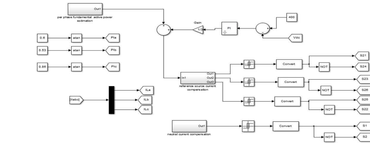
Fig: Matlab model of Shunt active power filter
